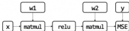
Figure 6: A simple dataflow graph example. Note: in this example, the MSE calculation has been represented as a single node. In actuality, MSE contains multiple operations that should be represented as separate nodes.
