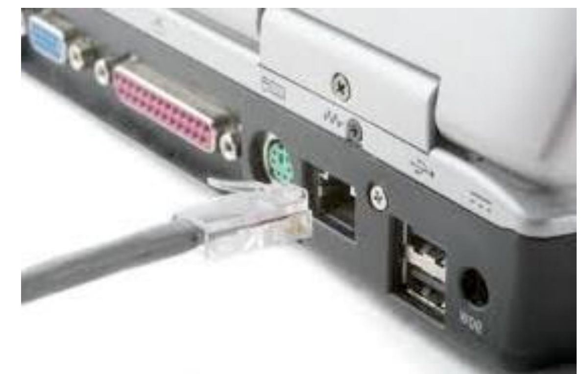
Ethernet cable and port
